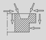
FFMM are modular portable machines for flange facing of large flanges. Mounted internally, they are used for different types of flange machining, making grooves for seals, preparation for welding or repair of the heat exchangers. They have a pneumatic drive and can machine flange diameter from 1200-5500 mm. All machines have a common turntable. According to requirements, the needed size of machine can be obtained by modification of the module.
