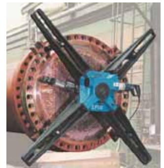
EFCO TDF-2 flange turning work range \Phi 300-1200 mm mounting \Phi 480-1380 mm
