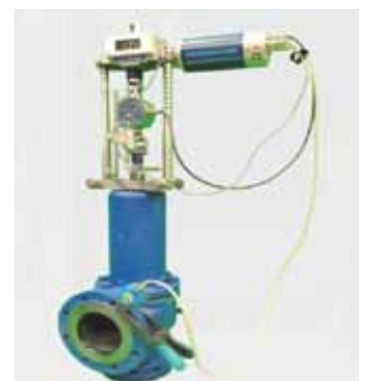
LEGATEST on-site testing and adjustment of safety valves
