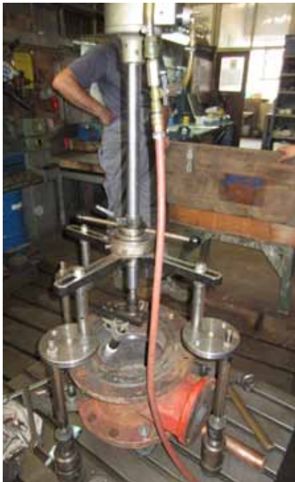
High speed grinding of valve seat
