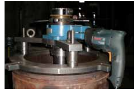
Turning the valve seat at the depth 1150 mm
