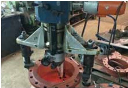
Turning the seat of the non-return flap
