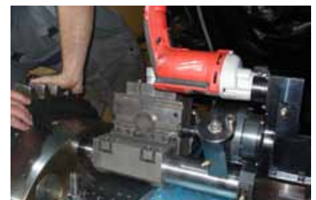
Turning a bore on a coupling turbine - generator
