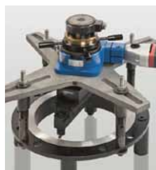
EFCO TDF-1 flange turning work range \Phi 0-500 mm mounting \Phi 260-600 mm
